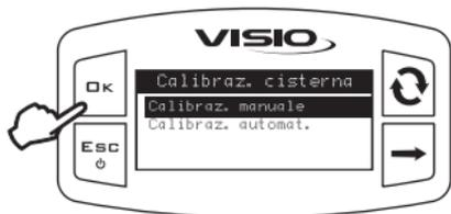
1) Open manual calibration menu (Setup menu > Tank > Man. Calibration).
