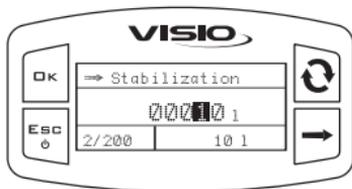
The message **Stabilization** will appear in the display top part for a few seconds, then it will switch back to **Rec. cal. point**.
