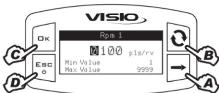
3) Set the Rpm constant value, i.e. the number of detection points, such as magnets or bolts fitted on the rotating shaft whose rotation speed shall be detected:
