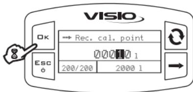
4) Once the tank has been emptied completely, press **OK** key for 1 second to complete the calibration process and save the relevant curve.
